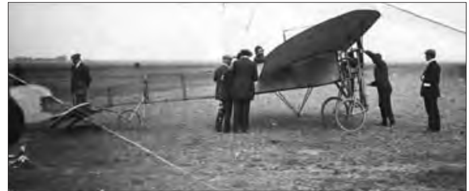
Designing “by eye” and without any attempt at systematization, Louis Blériot was able to increase curvature over the forward part of the wing section of his historic number 11 airplane. The added wing camber in that location helped the airplane to make its historic crossing over the English Channel in 1909. National Air and Space Museum, Smithsonian Institution (SI 78-14792)
