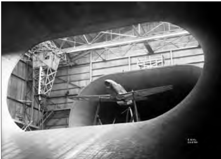
The NACA put the Mustang through systematic drag reduction tests in Langley's Full Scale Tunnel. NASA Image #L-34590 (LaRC)
