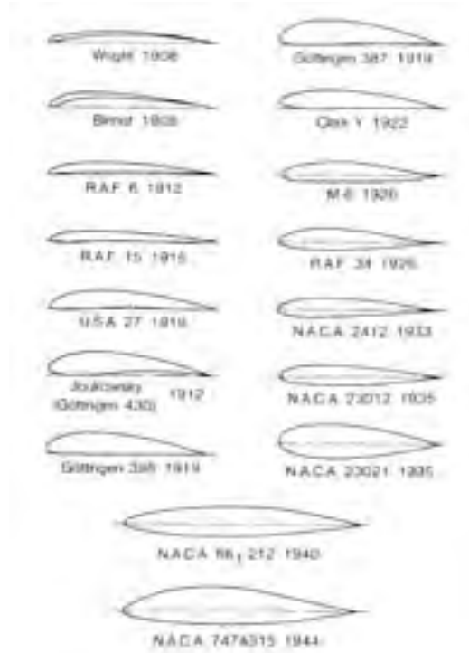
The historical evolution of airfoil sections, 1908-1944. The last two shapes are NACA low-drag sections designed to have laminar flow over 60 to 70 percent of chord on both the upper and lower surface. NASA Image #L-1990-04334 (LaRC)
