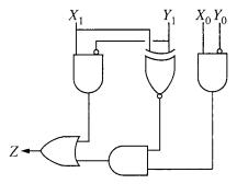
The logic circuit above is used to compare two unsigned 2-bit numbers,  $X_1 X_0 = X$  and  $Y_1 Y_0 = Y$ , where  $X_0$  and  $Y_0$  are the least significant bits. (A small circle on any line in a logic diagram indicates logical NOT.)
