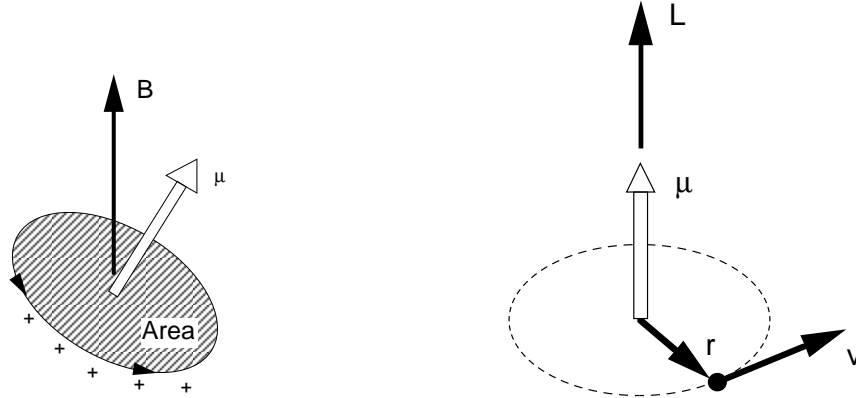
Fig. B.3. A current loop in magnetic field. A particle in a closed orbit.
