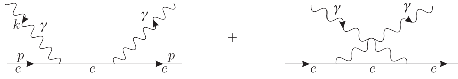
Fig. 2.2. Amplitude for e^\pm + \gamma \rightarrow e^\pm + \gamma . k is the photon 4-momentum and p that of the electron.
