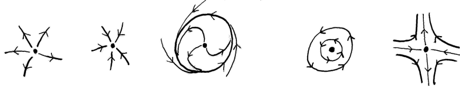
Figure 1.3. Fixed points in a two dimensional phase space: a source, a sink, a limit cycle, an elliptic fixed point, and a hyperbolic fixed point.
