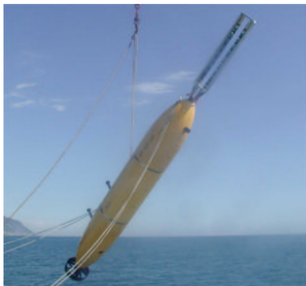
Figure 4.2: An autonomous underwater vehicle about to be launched. The large fork on the front is a sonar designed to detect buried mines. Within the hull is a transceiver which emits a “call” pulse into the water column. Beacons deployed at known locations detect this pulse and reply with a “acknowledge” pulses which are detected by the transceiver. The difference in time between “call” and “acknowledge” is proportional to the distance between vehicle and each beacon. (photo courtesy of MIT) see figure 4.2.2
