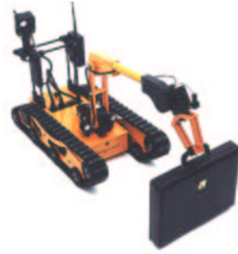
Figure 2.4: A vehicle with a high dimensional configuration space - a commercial bomb-disposal platform (picture courtesy of Roboprobe Ltd. The configuration space for a human is immensely high dimensional —around 230.
