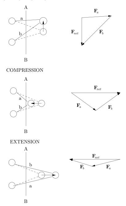
Figure 2.2. Relation between displacement and force on a molecule.
