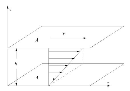
Figure 8.1. Sketch of experiment to determine the resistance of a fluid to shearing deformation.
