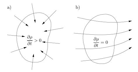
Figure 3.3. Illustration of a) divergent (actually, convergent) and b) nondivergent flow.
