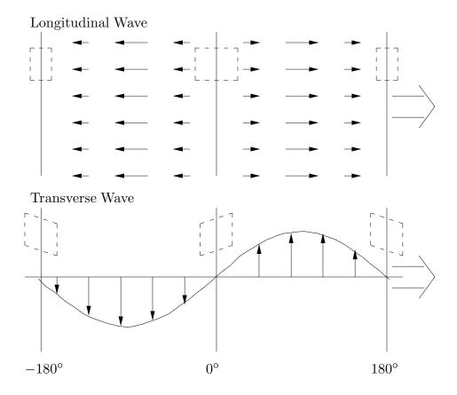
Figure 6.1. Displacement fields for longitudinal and transverse waves moving to the right. The dashed boxes show how an initial cube of material is deformed.
