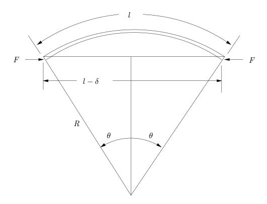
Figure 7.6. Sketch of relationship between the effective shortening,  $\delta$ , of a beam undergoing buckling, and the radius of curvature, R, of the beam.
