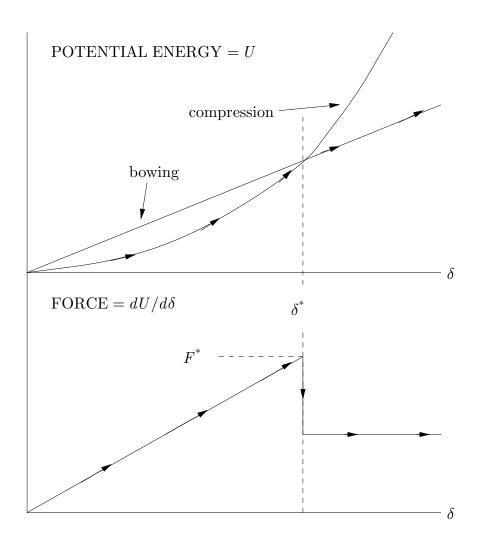
Figure 7.7. Potential energy of a beam shortened by an amount  $\delta$  under the influence of compressive forces on the ends, and the force required to maintain this reduction in length. Note that at the transition from compression to buckling at  $\delta = \delta^*$ , the required compressive force drops by a factor of two.
