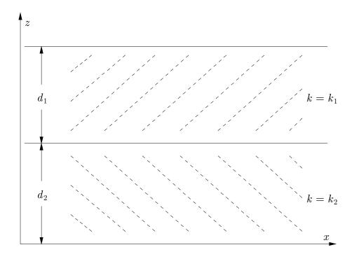
Figure 9.4. Two horizontal layers of soil with differing thickness and permeability. (See problem 7.)
