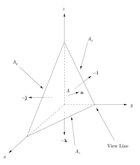
Figure 2.4. Definition sketch of tetrahedron used to derive the traction across an arbitrary surface from the tractions across three mutually perpendicular surfaces.
