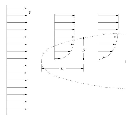
Figure 8.4. Initially uniform flow past a flat plate aligned with the flow. A boundary layer forms next to the plate, in which the fluid velocity is reduced from its initial value. The boundary layer thickens with increasing distance behind the leading edge of the plate.
