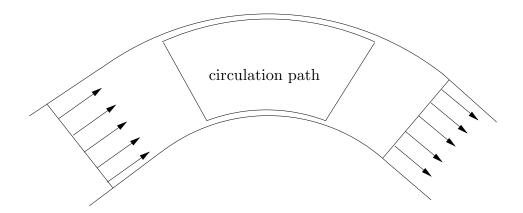
Figure 10.10. Water flowing irrotationally in a curved channel.
