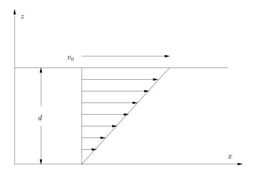
Figure 9.1. Creeping flow between two parallel plates, one of which is moving.
