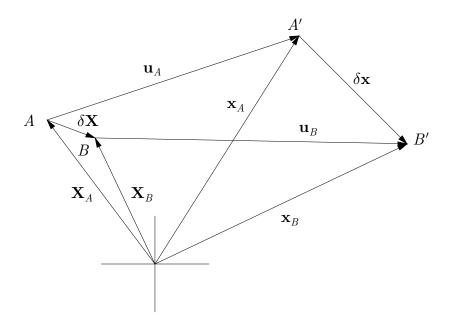
Figure 4.1. Relationship between the displacements of two parcels, A and B.
