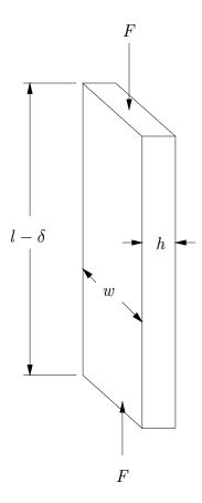
Figure 7.5. Definition sketch for buckling calculation.
