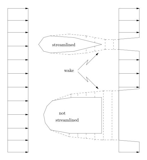
Figure 10.6. Development of a wake behind streamlined and unstreamlined bodies.
