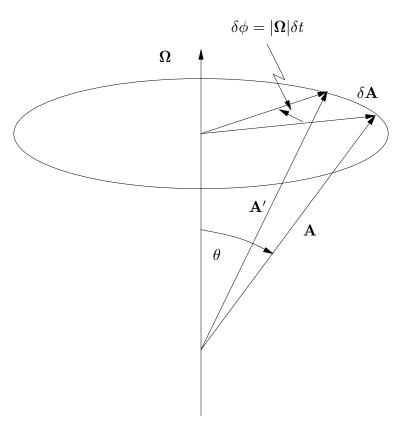
Figure 3.5. Definition sketch for relating the components of a vector in stationary and rotating reference frames.
