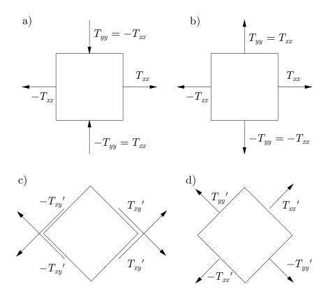
Figure 2.7. Tractions on edges of a square in two different cases, a)  $T_{yy} = -T_{xx}$ , and b)  $T_{yy} = T_{xx}$ , with  $T_{xy} = T_{yx} = 0$ . When the square is rotated by 45°, c) and d) show the transformed tractions.
