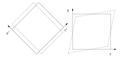
Figure 4.3. Effect of strain on two squares rotated 45° relative to each other.
