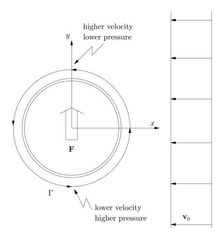
Figure 10.8. Lift acting on a rotating cylinder.
