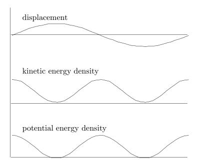
Figure 6.2. Relationship between wave displacement kinetic and potential energy densities in an elastic wave.
