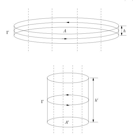
Figure 10.5. Illustration of "vortex stretching". The dashed lines are vortex lines.
