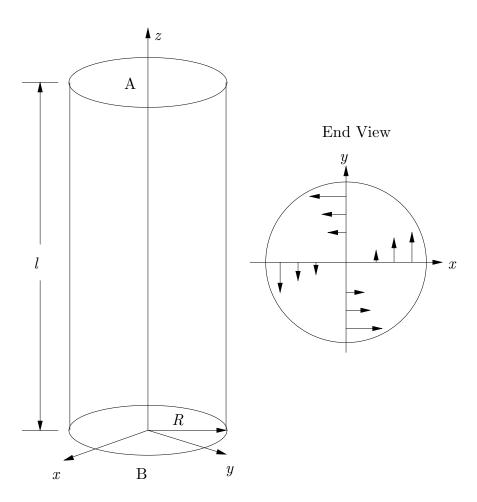
Figure 7.1. Definition sketch for torsion applied to ends of a cylinder.
