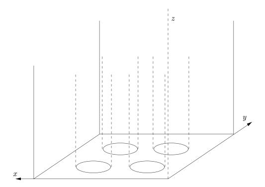
Figure 9.3. Flow through a porous medium idealized as flow through a parallel array of pipes.
