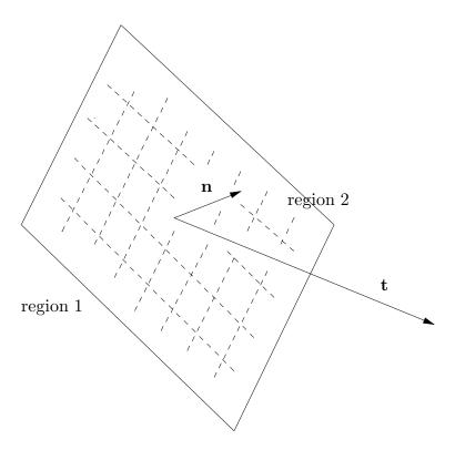
Figure 2.3. Illustration of the traction (t) and unit normal (n) vectors relative to a surface cutting a continuous medium. The traction is the force per unit area of region 2 acting on region 1.
