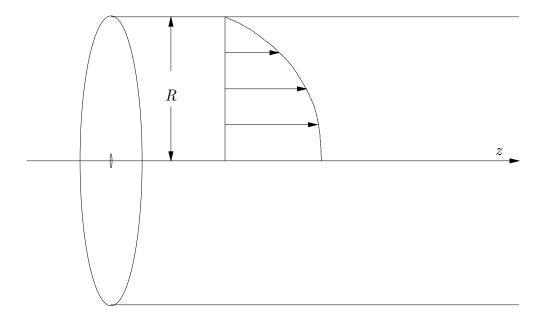
Figure 9.2. Sketch of laminar flow through a pipe of radius R.
