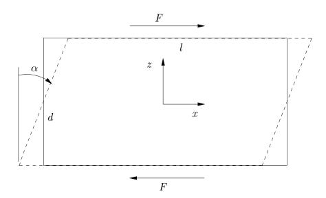
Figure 5.2. Deformation of a rectangular parallelepiped under the influence of shear tractions.
