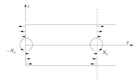
Figure 7.3. Tractions occurring at the ends and across a surface normal to a beam that is undergoing bending. The tractions result in a torque (or bending moment) in the y direction.
