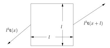
Figure 3.1. Definition sketch for computing the force imbalance on a cube. On the left side of the cube, the force is  $l^2\mathbf{t}(x) = -l^2[T_{xx}(x)\mathbf{i} + T_{xy}(x)\mathbf{j} + T_{xz}(x)\mathbf{k}]$ , while on the right side, it is  $l^2\mathbf{t}(x+l) = l^2[T_{xx}(x+l)\mathbf{i} + T_{xy}(x+l)\mathbf{j} + T_{xz}(x+l)\mathbf{k}]$ .
