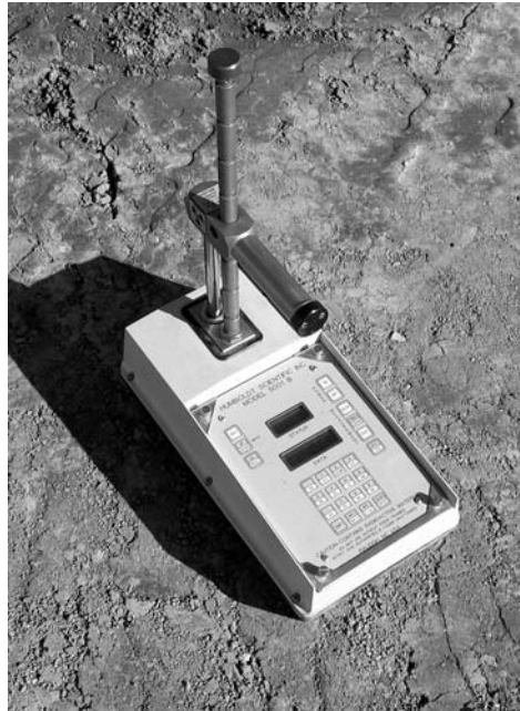
Figure 13.18 Nuclear density gauge. For transmission measurements the probe is lowered the desired distance into a hole previously prepared in the soil. (Photo courtesy Dr. David White.)
