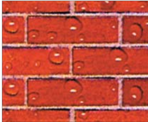
Waterproofing by Silicon Based Water Repellant Material.
