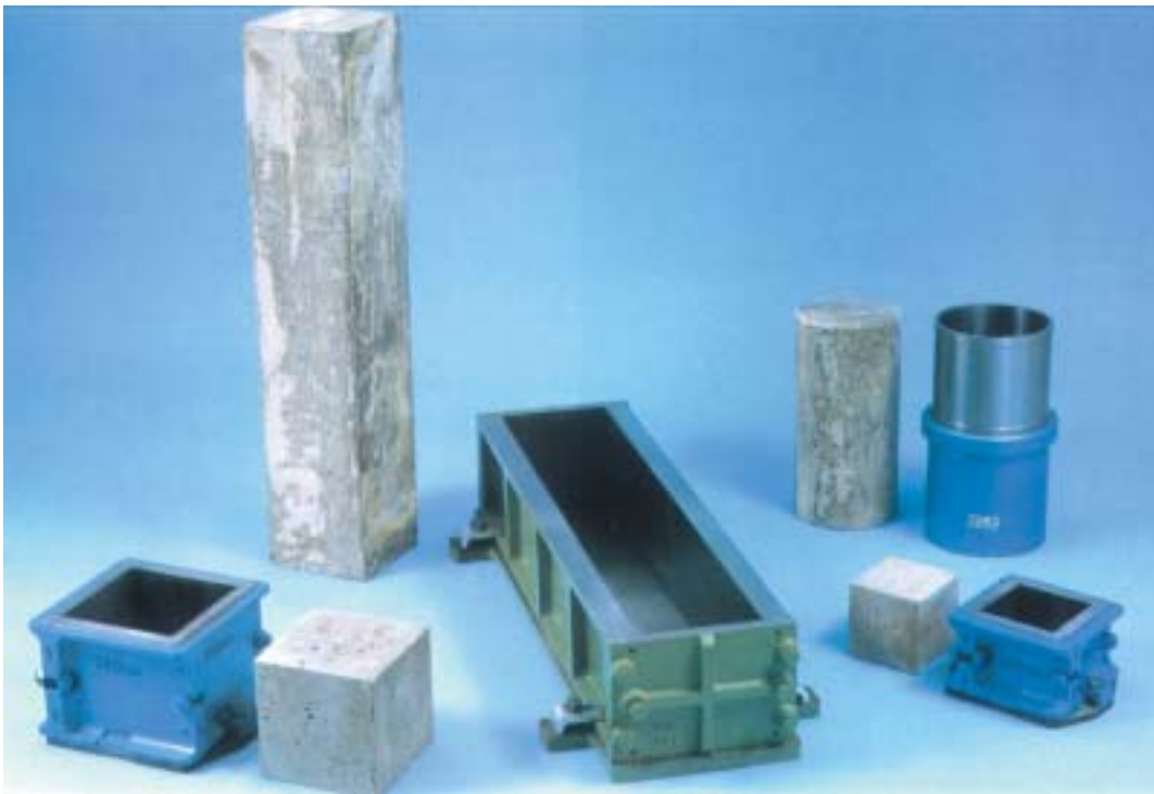
Cube beam and cylinder moulding
