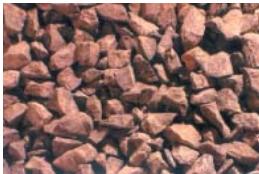
20 mm crushed angular aggregates not so good for concrete.
