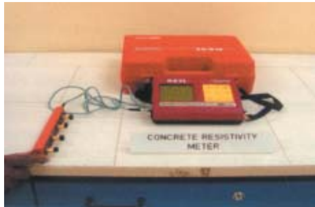
A view of Resistivity meter well connected with Wenner four probe, ready to measure the resistivity of concrete.
