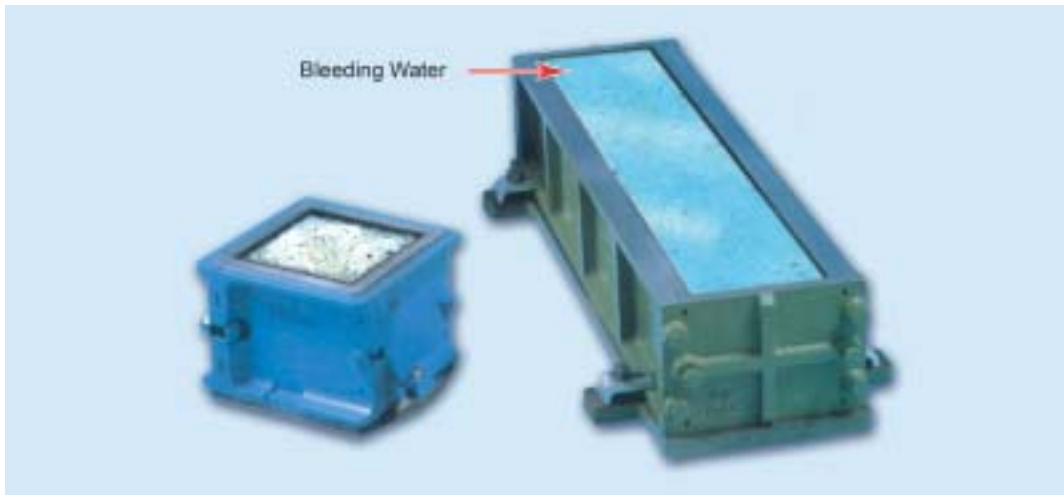
Example of external bleeding
