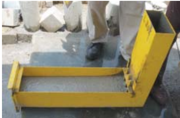
Concrete flowing through L-Box Courtesy : Hindustan Construction Company
