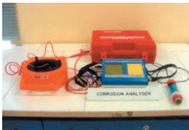
A view of Corrosion Analyser for half-cell potential measurement with the help of copper/copper sulphate reference electrode.
