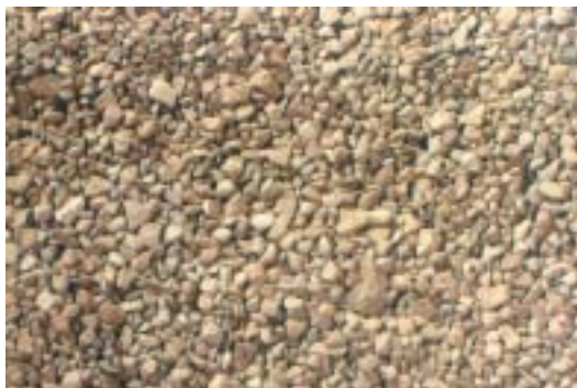
Good aggregate resulted from Barmac crusher.
