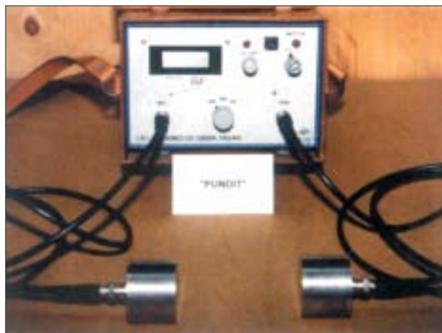
Ultra Sonic Pulse Velocity Equipment is used for finding dynamic modulus of elasticity.
