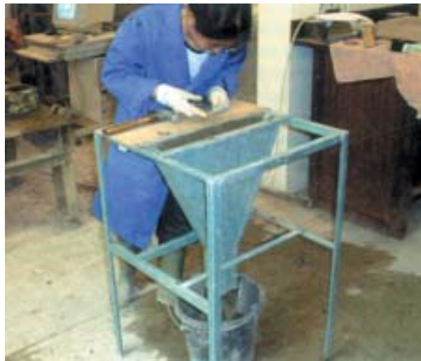
Observing the time of emptying of concrete from V-funnel.
