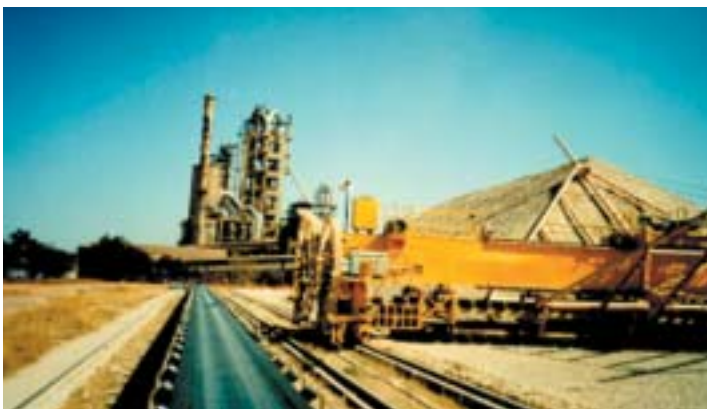
Reclaimer for homogenization of crushed limestone.
