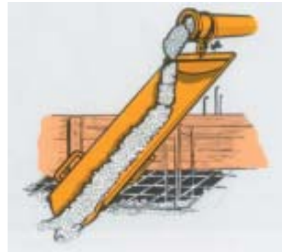
Transporting and placing concrete by chute.
