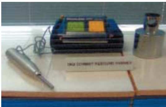
A view of Rebound Hammer connected with digital recording monitor and Test Anvil for calibration.
