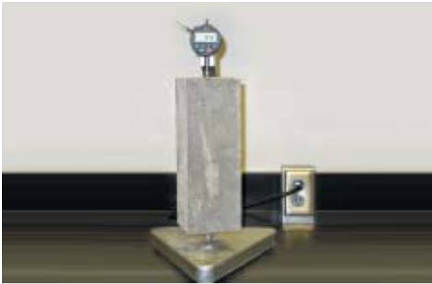
Length Comparator with specimen in place
