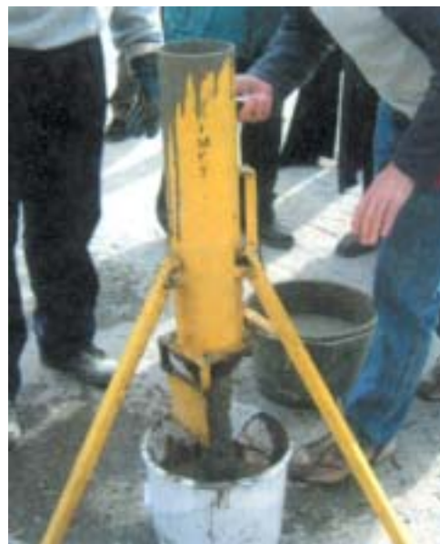
Concrete flowing through Orimet device
