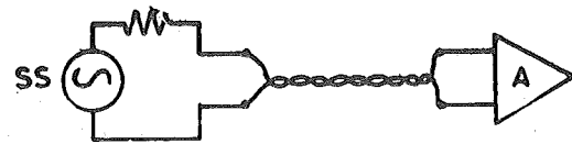
Fig. 43.4. Twisted pair of signal lead and floating apparatus input gives considerable noise immunity.
