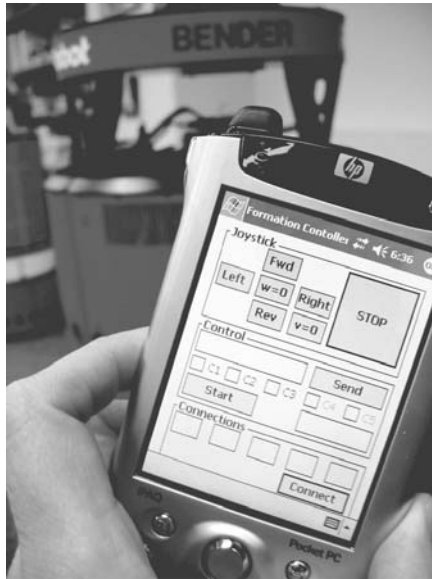
Fig. 5. Formation controller interface. A number of user interface screens like the one shown here have been created. The boxes labeled C1 through C5 allow the user to specify which robot (s)he wishes to communicate with.
