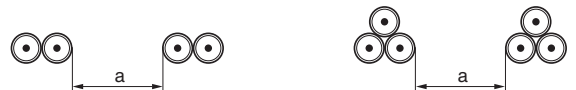
Fig. G18 : Reduction factors for more than one circuit, single-core or multi-core cables laid directly in the ground. Installation method D. (table 52-18 of IEC 60364-5-52)
