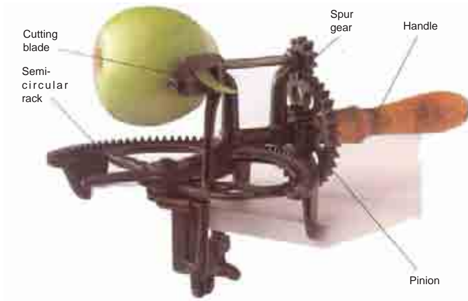
Kitchen Gear: This 1863 fruit and vegetable peeling machine uses a rack and pinion to drive spur gears that turn an apple against a cutting blade. As the handle is pushed round the semi-circular base, the peel is removed from the apple in a single sweep.
