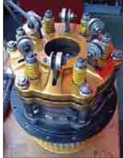
Centrifugal clutch with three discs and four steel float plates.
