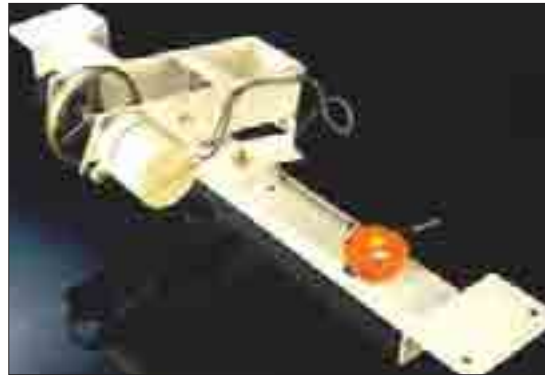
Belt slip indicator is used to indicate that the belt is slipping.
