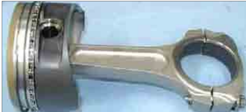
Piston rod is made of mild steel.
