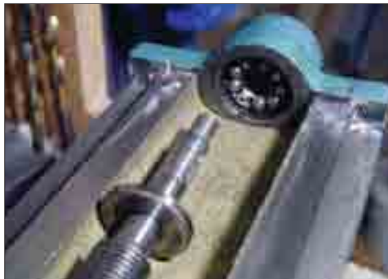
Lead screw supported by collar bearing.
