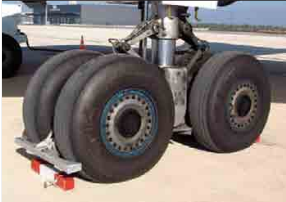
Aircraft landing gear is especially designed to absorb shock and energy when an aircraft lands, and then release gradually.
