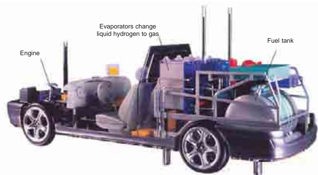
This experimental car burns hydrogen fuel in an ordinary piston engine. Its exhaust gases cause no pollution, because they contain only water vapour.
