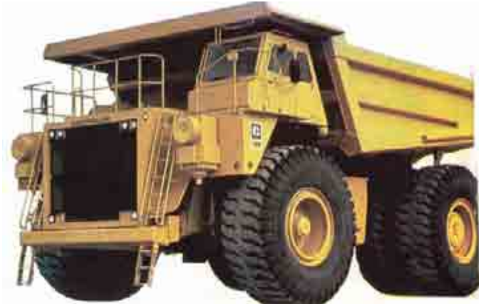
A mammoth caterpillar dump truck for use in quarries and open-cast mines.
