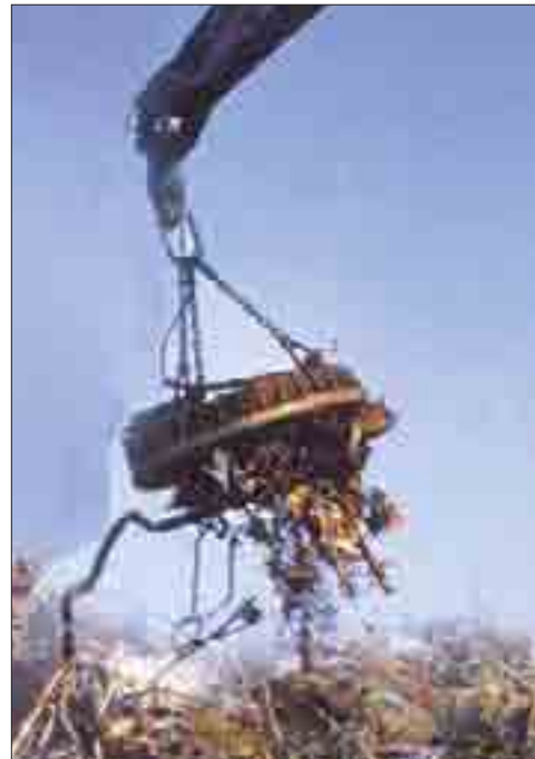
A large disc-shaped electromagnet hangs from jib of this scrapyards crane. Steel and iron objects fly towards the magnet when the current is switched on. In this way, iron and steel can be separated for recycling.
