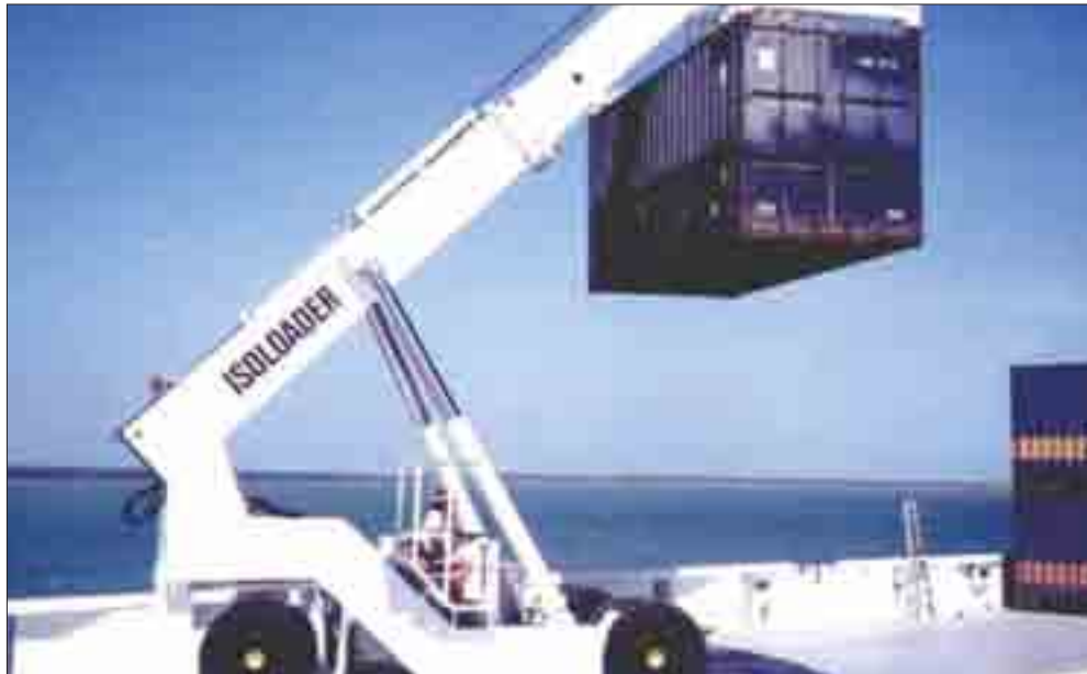
Deck-handler crane is used on ships to move loads
