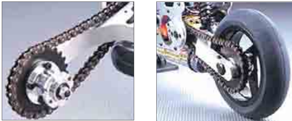
Rear wheel chain drive of a motorcycle
