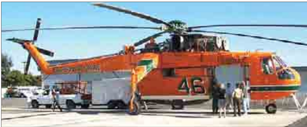
The propeller shaft of this heavy duty helicopter is subjected to very high torsion.
