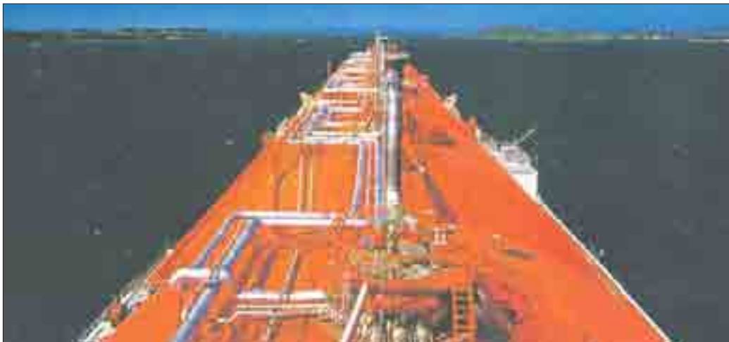
This view along the deck of a liquefied natural gas (LNG) carrier shows the tops of its large, insulated steel tanks. The tanks contain liquefied gas at -162°C.
