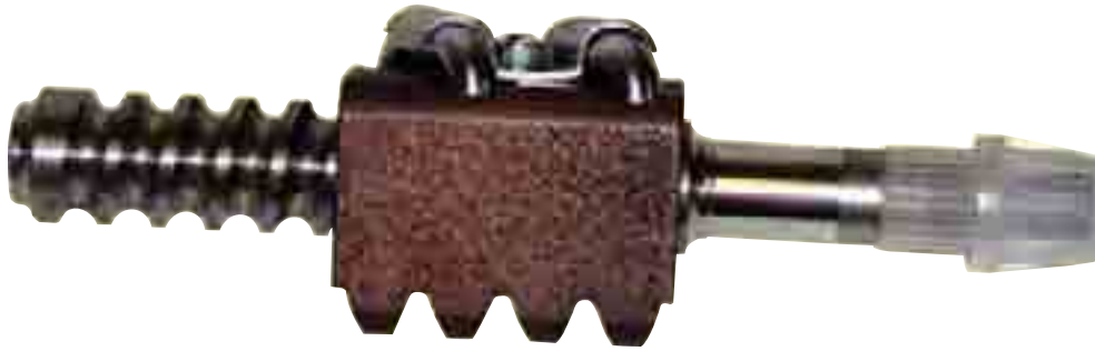
Worm gear of a steering mechanism in an automobile.
