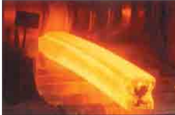
Hot Rolling : When steel is heated until it glows bright red, it becomes soft enough to form into elaborate shapes.
