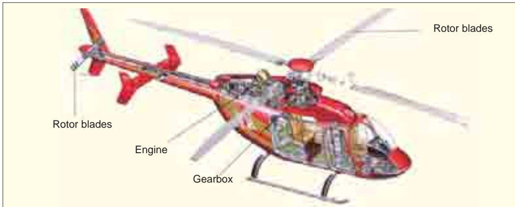
Air accelerating downwards, pushed by the rotating blades, produced an upwards reaction that lifts the helicopter.
