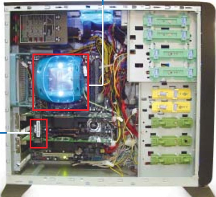
The bridge that connects the two SLI cards
