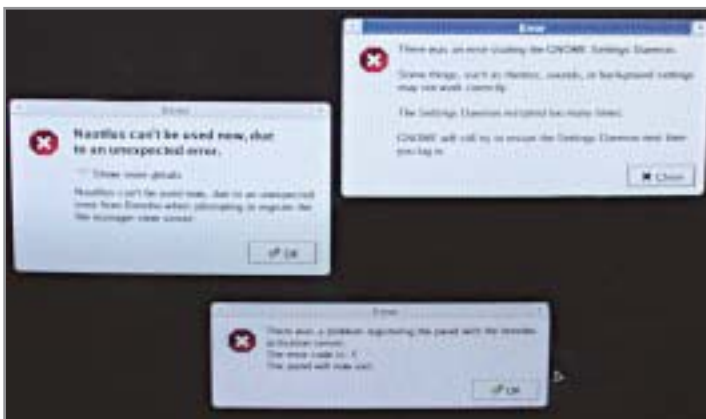
The moment you change the date of your Linux system to 2038, many applications crash and messages like the ones shown above pop up
