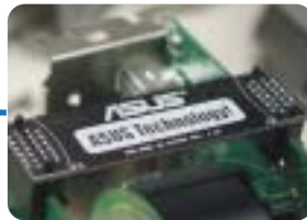
The bridge that connects the two SLI cards
