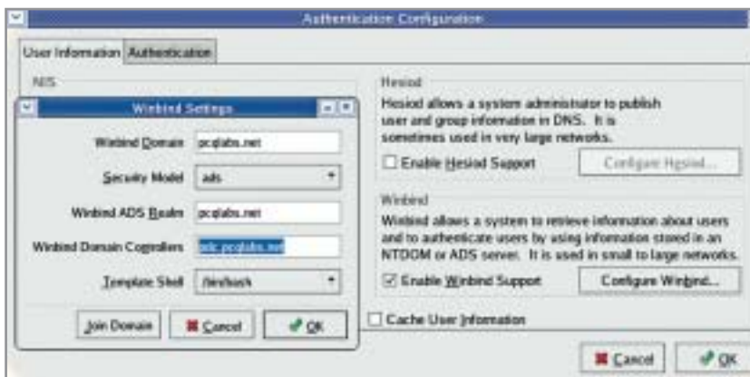
Samba can now be configured with WinBind authentication that allows it to connect to Windows Active Directory Servers
