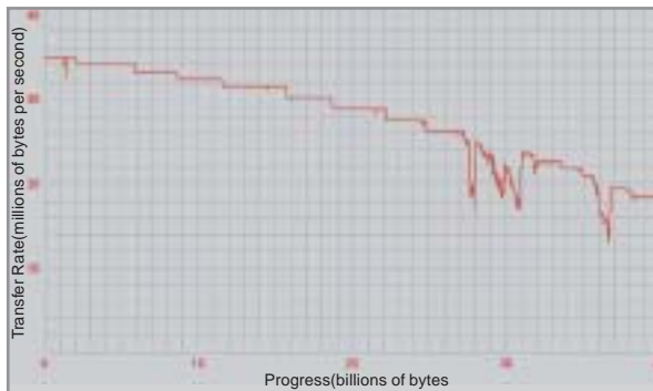
Notice how the throughput drops as you move from the outer circle to the inner circle of the hard disk platter
