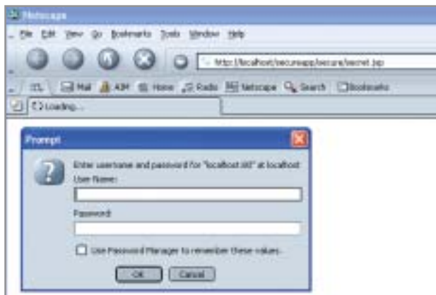
When access is restricted to a resource, Tomcat server causes an automatic authentication request to the remote browser
