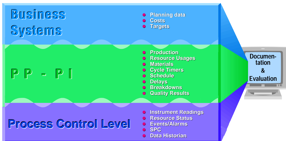
Fig. 11-1: Process data on different enterprise levels
