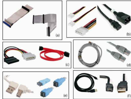
Figure F.2 Accessories – cables and connectors. (a) IDE cable connectors, (b) Power cables, (c) SATA cables, (d) CAT5 cables, (e) USB connectors, (f) USA A to mini-B connectors.
