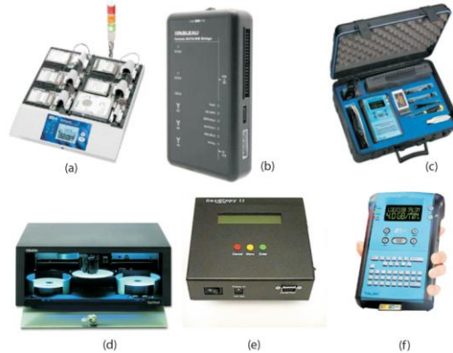
Figure F.1 Tools and equipment in computer forensics laboratory. (a) Wiping equipment, (b) Write protection equipment, (c) Portable forensics kit, (d) Archiving equipment, (e) Duplication equipment, (f) Data capturing device (handy model).
