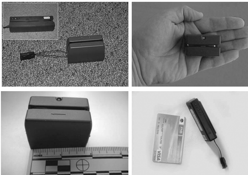
Figure 11.8 | Credit card skimmer devices.
