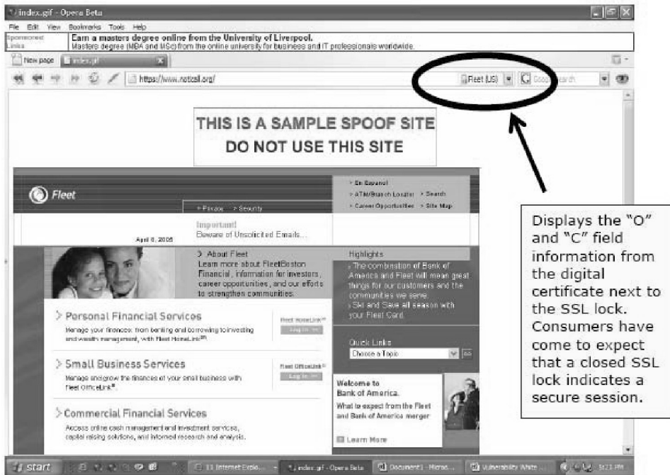
Figure 11.13 | Site with misleading organization name. Note: The color version of the figure is also available in the CD.
