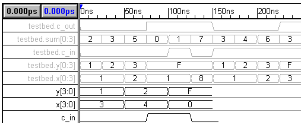
Figure 2: Stimulus vectors for the 4-bit adder circuit
