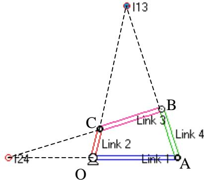
The instant center is defined as a point in which the two links have the same velocity. For a four-bar linkage, the instant center of the two conjunct links is the point at the pin joint between them; the instant center of the two opposite links, such as link 1 and link 3, is solved by the following method.
