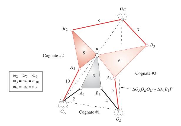
Find the three equivalent geared fivebar linkages for the three fourbar cognates in Figure 3-25a (p. 125). Check your results by comparing the coupler curves with programs FOURBAR and FIVEBAR.
