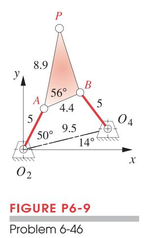
6-46 Figure P6-9 shows a linkage in one position. Find the instantaneous velocities of points A, B, and P if link  $O_2A$  is rotating CW at 40 rad/sec.
