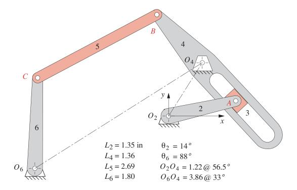
7-52 Figure P7-22 shows a mechanism with dimensions. Use a graphical method to calculate the accelerations of points A, B, and C for the position shown.  $\omega_2 = 20$  rad/sec.
