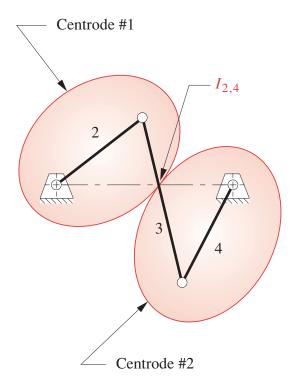
†9-61 Calculate and plot the train ratio of a noncircular gearset, as a function of input angle, that is based on the centrodes of Figure 6-15b (p. 290). The link length ratios are  $L_1/L_2 = 1.60$ ,  $L_3/L_2 = 1.60$ , and  $L_4/L_2 = 1.00$ .
