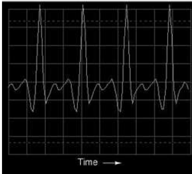
Figure 7.27: Oscilloscope display: waveshape of a trumpet tone.
