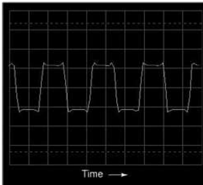
Figure 7.31: Oscilloscope time-domain display of a square wave
