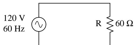
Figure 11.1: Ac source drives a purely resistive load.
