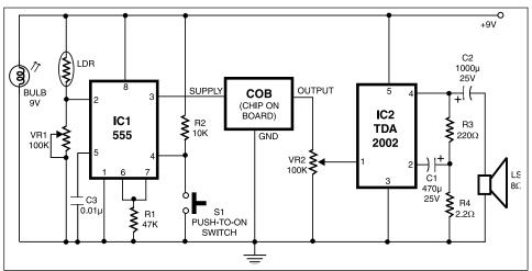
ever, one may select a COB which generates sound such as '*aag lag gai hai*'. The signal generated by COB is amplified by an audio amplifier. In this circuit, the audio power amplifier is wired around IC2 TDA 2002.
