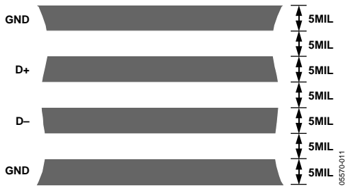
Figure 22. Typical Arrangement of Signal Tracks
