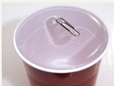
Surface tension prevents a paper clip from sinking.
