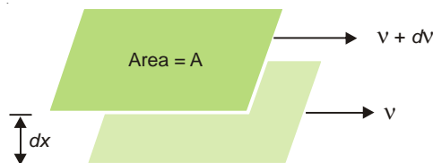
■ Figure 11.23 Two parallel layers moving in a liquid.
