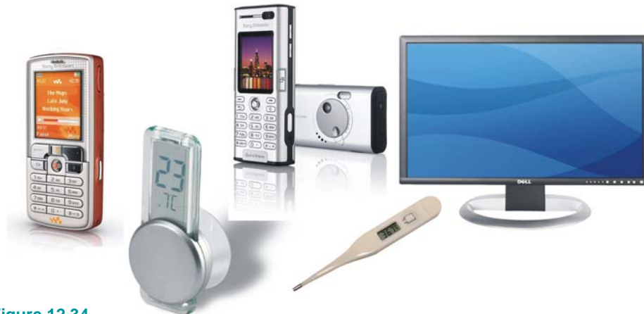
■ Figure 12.34 The technical application of liquid crystals in flat panel displays for desktop and notebook-computers or in the displays of cellular phones has become an indispensable part of modern information and communication technologies.
