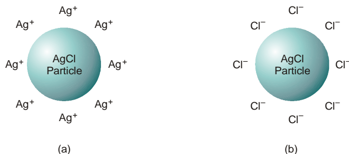
■ Figure 22.23 (a) When Ag + ions are in excess, AgCl sol particle adsorbs these ions and becomes positive; (b) when Cl - ions are in excess, the AgCl particle adsorbs these and acquires a negative charge.
