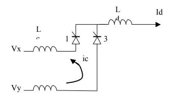
Assume that the dc smoothing inductor is so large that  $I_d$  may be considered constant. Assume thyristor 1 conducts. As thyristor 3 gets a firing pulse, the current starts commutating from thyristor 1 into thyristor 3.
