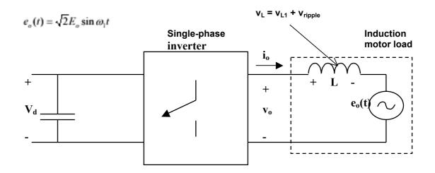
The problem with ripple in the output current from a single-phase full bridge converter is to be studied. The first harmonic of the output voltage is given by  $V_{o1}$  at f = 47 Hz. The load is given in the figure as L = 100 mH in series with an ideal voltage source  $e_o(t)$ . It is assumed that the converter works in square wave mode.
