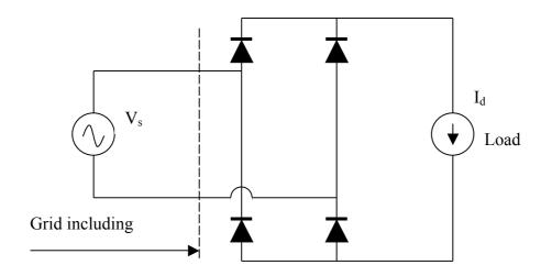
A single-phase diode rectifier with a current source as load.
