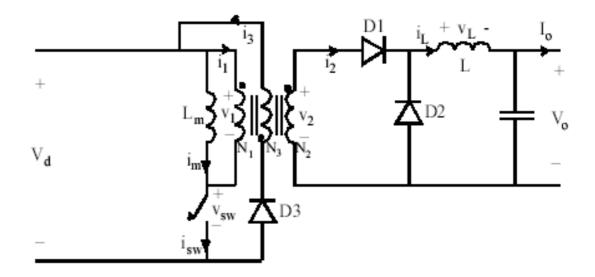
$\begin{array}{lll} V_d = 300 \; V & V_o = 6 \; V & f_s = 100 \; kHz \\ N_1 : N_3 = 1 & L_m = 15 \; mH & L = 0.05 \; mH \end{array}$
