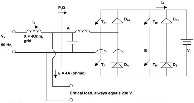
The figure over shows a converter, which charges a battery. It also holds the critical load voltage stable at 230 V. (In case of grid failure, the converter will work as an inverter. See figure 11-12).
