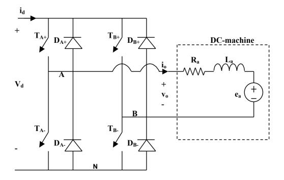
$V_{\rm d}$  = 250 V. Switching frequency is 30 kHz. The bridge is connected to a speed controlled dc machine. The armature inductance  $L_{\rm a}$  = 0,2 mH. The armature resistance is negligible.
