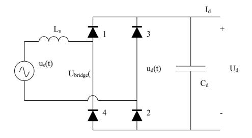
The figure shows a single-phase full bridge diode rectifier connected to a smoothing capacitor  $C_d$ . Assume that the capacitance of the smoothing capacitor is so large that  $U_d$  may be considered to be constant (no ripple). The diode rectifier is connected to a grid with a sinusoidal voltage  $u_s$ , equal to 230 V (rms) with frequency equal to 50 Hz. The inductance of the grid  $L_s$  is equal to 1.22 mH.
