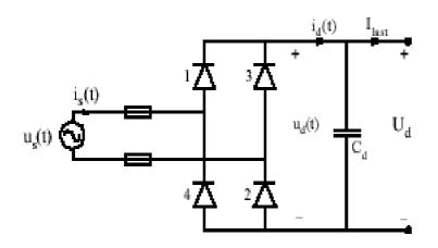
Diode rectifier with fuses
