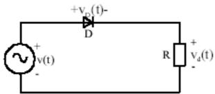
Given:  $v(t) = \sqrt{2} \times 230 \times \sin \omega t$ , where  $\omega = 2\pi 50$
