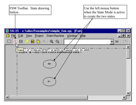
• To create a transition from state "s1" to state "s2", **select** the "Transition" button on the FSM Toolbar. To select state "s1", **click** and **release** with the left mouse button anywhere on the oval symbol for state "s1". Once state "s1" is selected, a small circle will appear on the state symbol for "s1" whenever the mouse cursor is near it.
