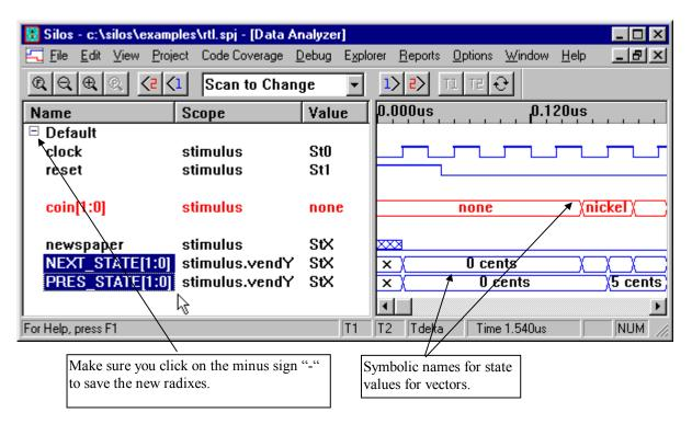
• Now use the "Set Radix" menu selection to set the radix for the vectors NEXT\_STATE[1:0] and PRES\_STATE[1:0]. To set the radix for both vectors at the same time, select both vectors by holding down the Ctrl key on the keyboard as you select them, and then use the "Set Radix" menu selection to change the radix. Make sure you click on the minus sign "-" for the default group to save the new radixes.
