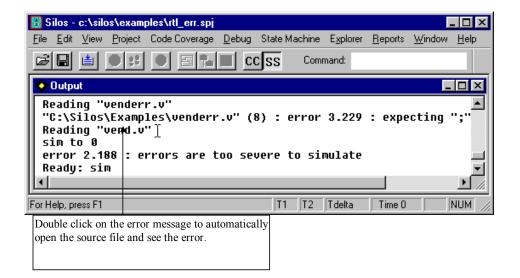
• **Double click** on the syntax error that is reported in the Output Window. This will open file "vend\_err.v" and highlight the syntax error. Notice that the real error occurred on the line above due to the missing semi-colon ";" for terminating the line. This is very common because Silos could not determine there had been an error until it got to the next line, where, instead of finding the module port list, Silos encountered a register statement.
