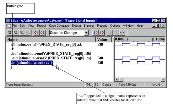
• Signal "stimulus.vendY.\PRES\_STATE\_reg[0].ck" is driven by a buffer whose input is "stimulus.\clock<c>". The "<c>" appended to the signal name "clock" means it is a wire created for internal use by the Silos program. This internal signal is used to represent the signal "clock" across the port boundary from module "stimulus" into module "vend".
