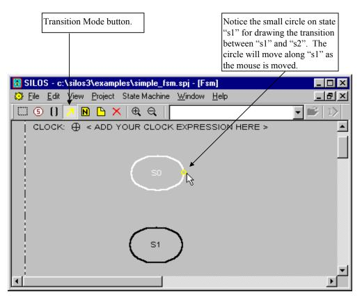
To draw the transition from state "s1" to state "s2", **position** the mouse cursor on the oval symbol for state "s1", **click** and **hold** down the left mouse button, and **drag** the mouse cursor from state "s1" to state "s2". When the mouse cursor gets near state "s2", an arrow will appear on the transition line. You can **release** the left mouse button after the arrow appears, and the transition between "s1" and "s2" is complete.
