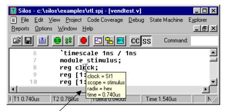
Data Tips display value, scope, radix, and simulation time point for variable clock. The time point can be set by the "T1" timing marker in the Data Analyzer. The Data Tips can be turned on/off and the radix can be changed by using the context menu in the source window.
