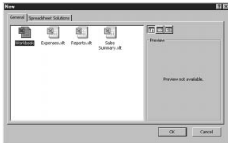
Figure 2.28. Excel looks for .xlt files in the Templates folder and all of its subfolders. It displays a tab for any folder found to contain an .xlt formatted file.
