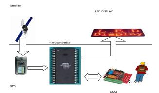
The main goal of this project is to design college bus location system, which will track the location of the bus using GPS. Due to security concerns, we will be using GPS system to monitor college buses to find approximate location of the bus and GPS location Of The bus status will be displayed at all the bus terminals using an LCD display
