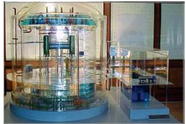
Fig 4: Scaled Model (1:50) of AHWR Acrylic Material
