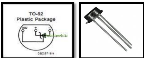
Fig. 9 connection digram of LM-236-5 reference diode
