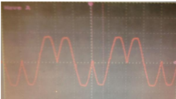
7.6 Fig output at load for frequency F=25\text{Hz} i.e F/2
