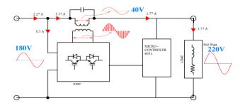
Fig: block diagram static voltage stabilizer (boost mode)
