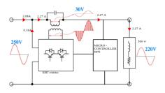
Fig: block diagram static voltage stabilizer (buck mode)
