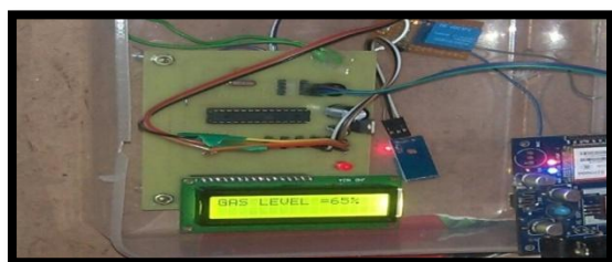
fig 1.1.8: LCD displaying gas level value
