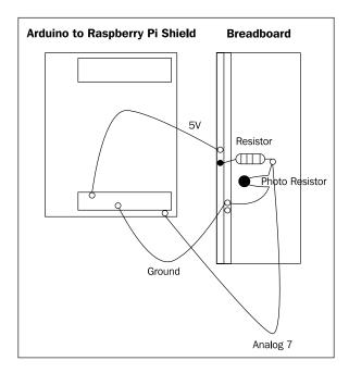
Now that we have the hardware in place, we can write an application to test our setup.
