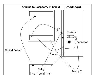
Finally, if your relay requires an external power supply, connect this. Your circuit, when connected, should look similar to the following diagram:
